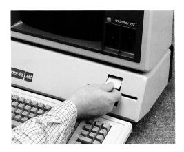
Figure 1-5. Opening the Disk Drive
